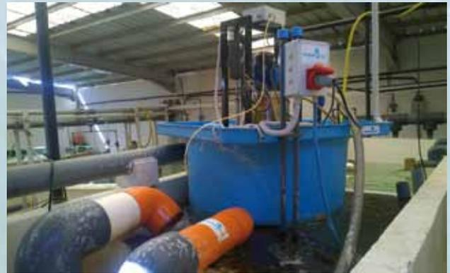
**Skim Plus** is a filtration control system by automatic foam adjustment.
